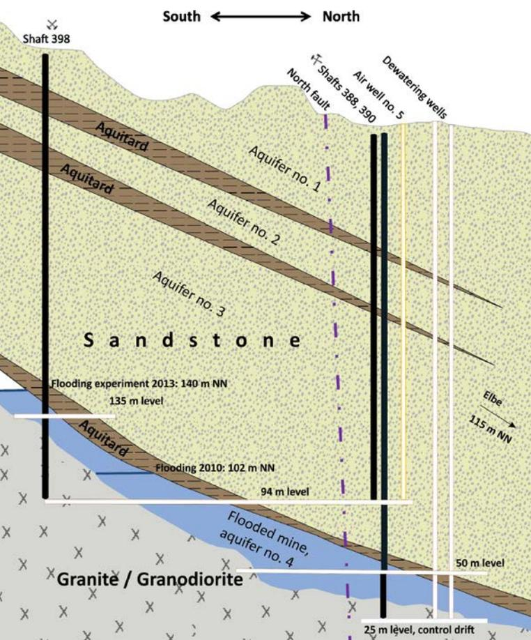
The flood monitoring network monitors the rise of the groundwater level in the third and fourth aquifers, the void subject to flooding, and the groundwater quality during and after flooding of the Königstein mine. Monitoring focuses on areas constituting zones of potential flood water rise to the third aquifer and on areas downstream of the third and fourth aquifers along the northern and western edges of the mine.
