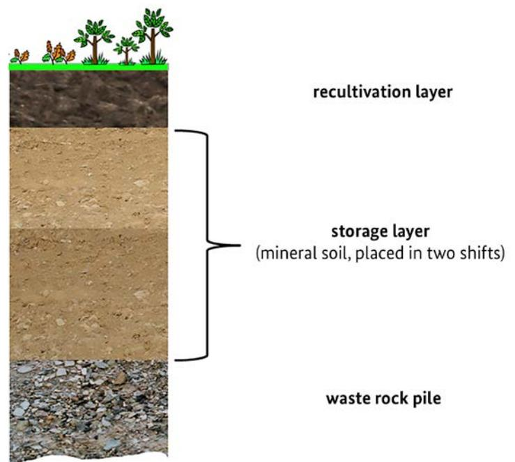
(which serve as drainage materials). Once the earthworks are completed, grass and herb mixtures are sown. This primary seeding serves as protection against erosion and stabilises the newly established topsoil layer.
