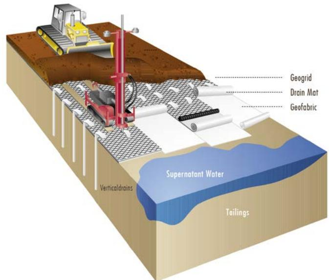
step, the supernatant water is gradually removed from the tailings ponds and treated in water treatment plants. Finally, the exposed sludges are subjected to an additional technical drainage process, stabilised and finally covered.
