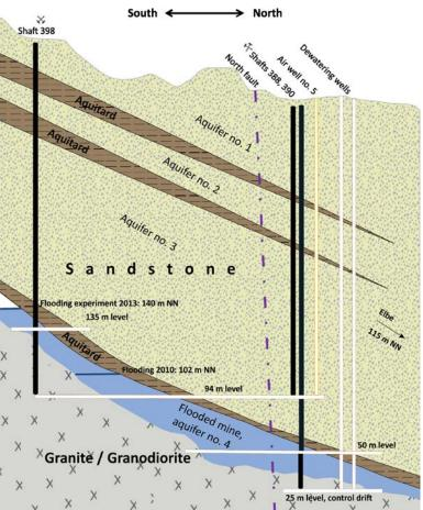
The flood monitoring network monitors the rise of he groundwater level in the third and fourth aquifers, the void subject to flooding, and the groundwater quality during and after flooding of the Königstein mine. Monitoring focuses on areas constituting zones of potential flood water rise to the third aquifer and on areas downstream of the third and fourth aquifers along the northern and western edges of the mine.
