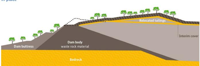
Figure 5: Standard profile of a contoured tailings management facility with the final cover in place
