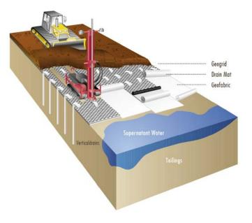
step, the supernatant water is gradually removed from the tailings ponds and treated in water treatment plants. Finally, the exposed sludges are subjected to an additional technical drainage process, stabilised and finally covered.
